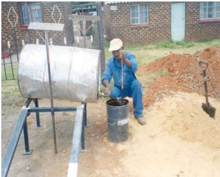
Photo 4.32: Stand for decanting binder
