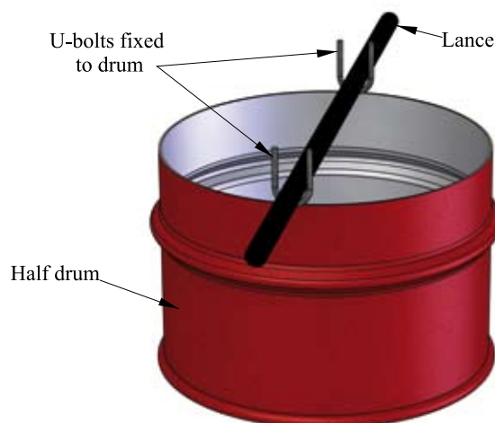
Figure 4.2: Rack for spray lance
